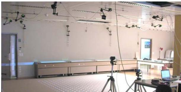
Figure 5. Motion capture area used for the study on stepping. Cameras are fixed to the wall, the ceiling or on tripods. On the ground one can see a video-projected calibrated pattern to guarantee the correct display of targets [15].
