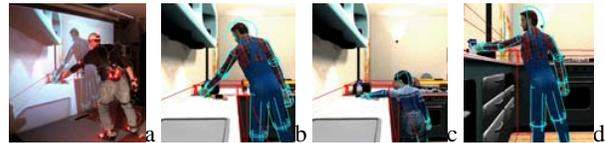
Figure 1. (a) immersive display with active marker motion capture system, (b) the controlled same-height avatar, (c) controlling a child avatar with the same visual scale as in a and b, (d) egocentric scaling strategy: the virtual environment is scaled as experienced by the child avatar [BMT09].
