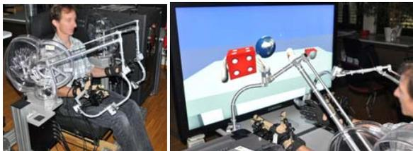
Figure 4. The user is seated in the haptic workstation (left); both the arms and the fingers can be guided by force feedback when manipulating an object (right). Physically-based interactions [14] exploit PhysX from Nvidia.
