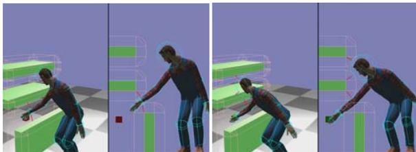
Figure 2. The posture of the virtual human avatar is driven by motion capturing the user [8]; the posture reconstruction is combined with collision avoidance owing to damping constraints (red lines) [7].
