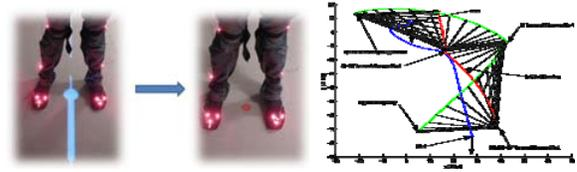
Figure 6. An example of videoprojected start location (left), the end location is constant in space (middle), measured step sequence (right).
